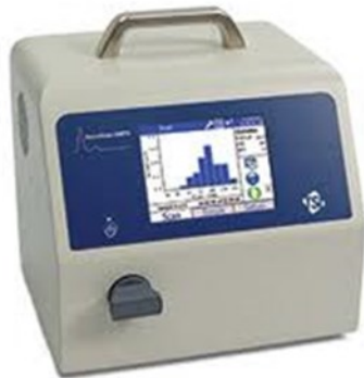
NanoScan SMPS 3910 - Portable sorter and counter of particles, size range 10-350 \mu\text{m}
